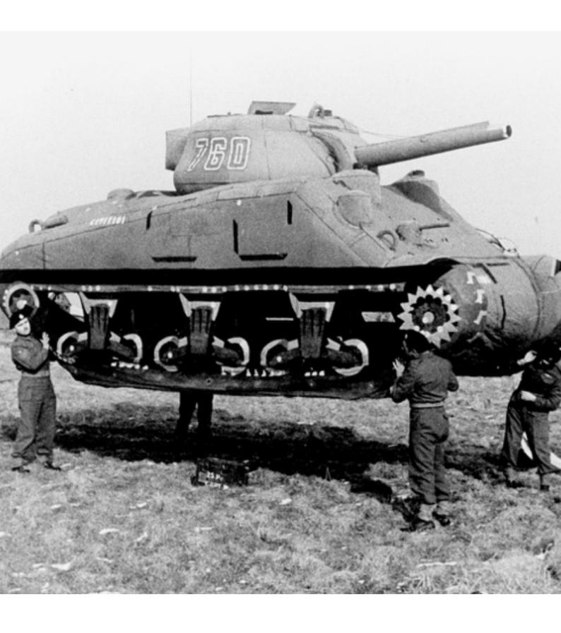
Figure. 6: Decoy Inflatable Tank
